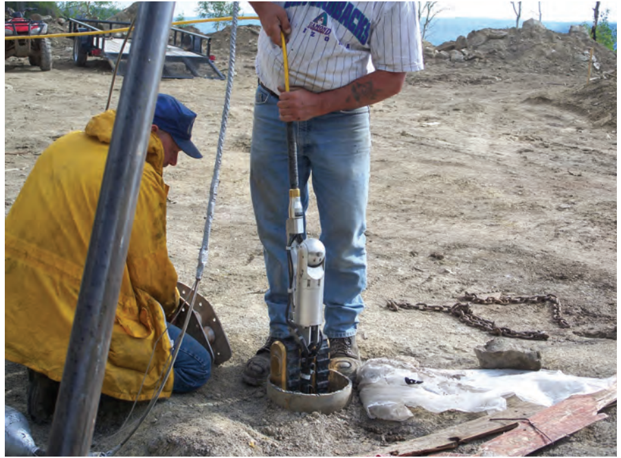
A camera robot being inserted in a bore hole at Crandall Canyon Mine in Utah.
